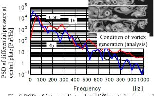
Fig.5 PSD of intermediate plate differential pressure by LES calculation
