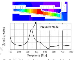
Fig.7 Acoustic calculation result of straightening plate by boundary element method
