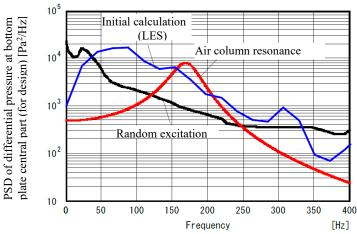
Fig.8 PSD for design of air column resonance and random excitation component (bottom plate central part)
