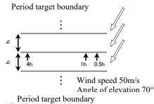
Fig.4 Fluid numerical analysis model
