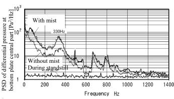
Fig.6 Differential pressure PSD of bottom plate central part by 1/3 scale model test
