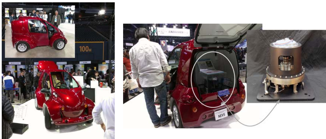
Fig. 8 A prototype electric vehicle for cold region (left) and magnetic heat pump system on board (right)
