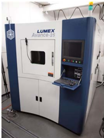
Fig. 10 A metal powder layering selective laser sintering machine (left:Lumex Avance-25 by Matsuura Machinery Corp.) and its product model of porous structure for AMR (right)
