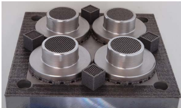
Fig. 10 A metal powder layering selective laser sintering machine (left:Lumex Avance-25 by Matsuura Machinery Corp.) and its product model of porous structure for AMR (right)
