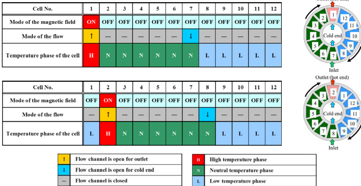
Fig. 7 A general schedule of heat exchange in a rotation disk of apparatus
