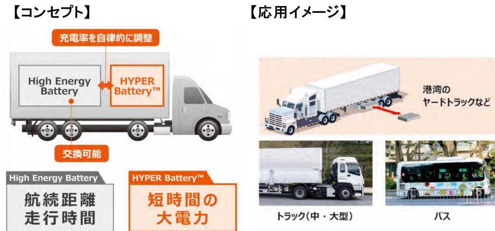
Fig. 4 Concept of Hybrid Battery for heavy duty vehicle
