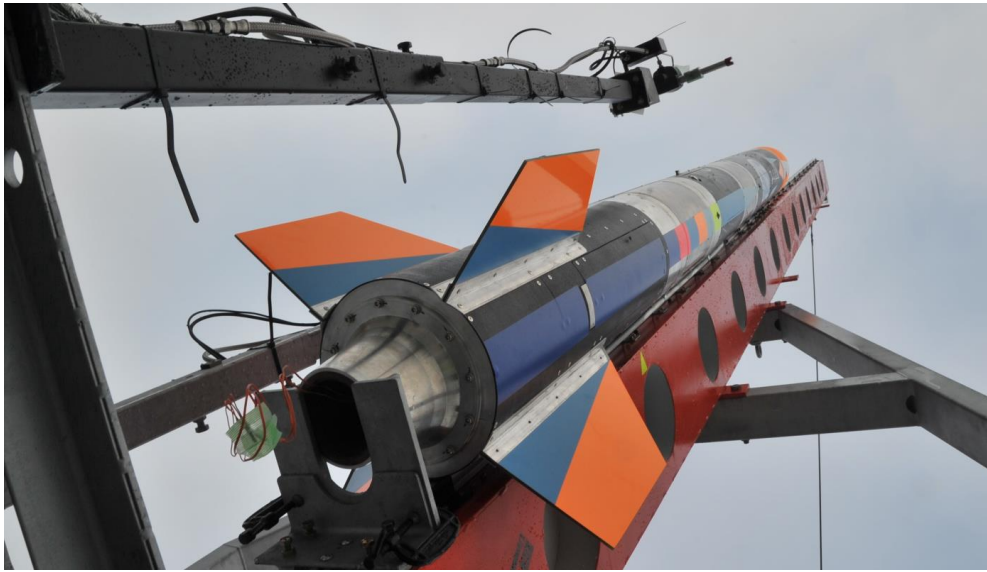
Fig. 8 The prototype of 500 kgf-class hypersonic rocket "Suzukaze", using pintle-type injector
