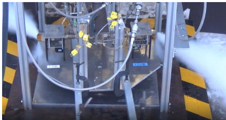
Fig. 6 Roll angle control experiment of sounding rocket with hot gasjet thruster
