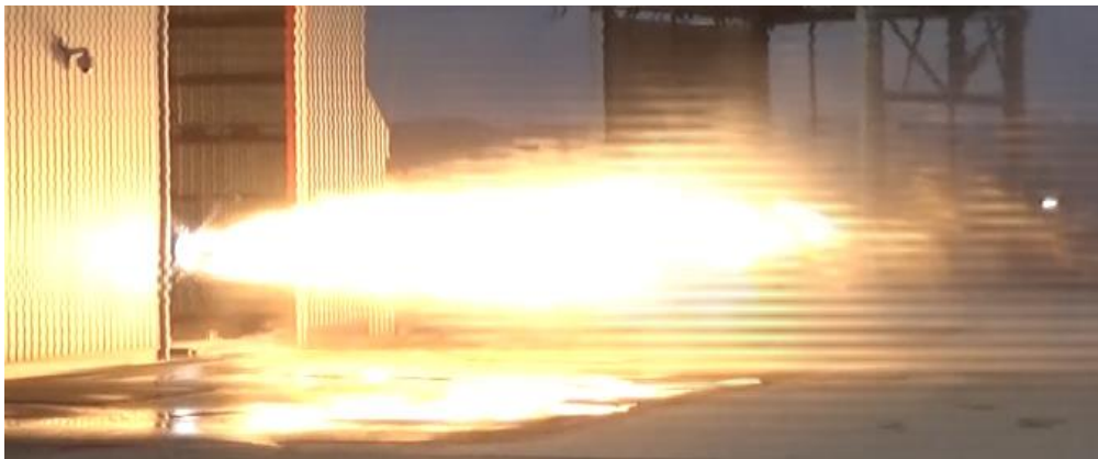
Fig. 9 Ignition of 6 tonf class pintle type engine with hydrocarbon fuel
