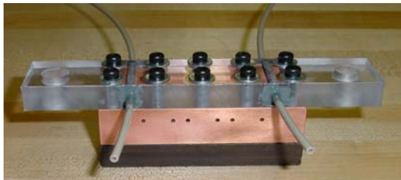
Figure 2 Flow visualization test section used by Kandlikar and Steinke (2003a) during flow boiling of water in 200 micron square microchannels.
