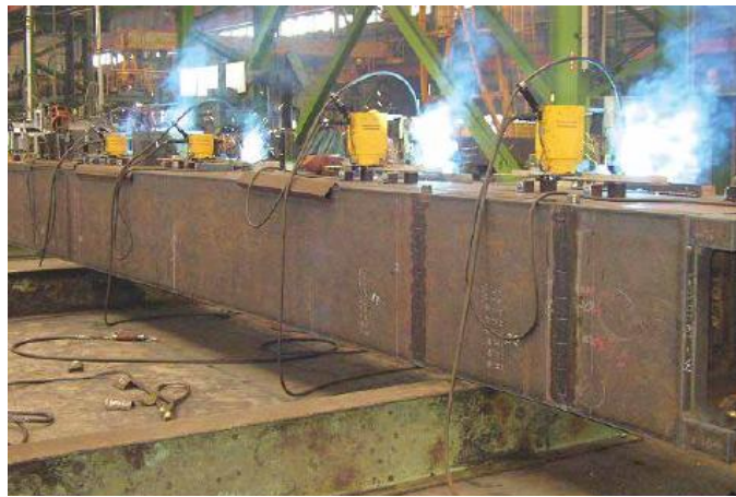
Figure 4. Example of multiple-units-per-operator application
