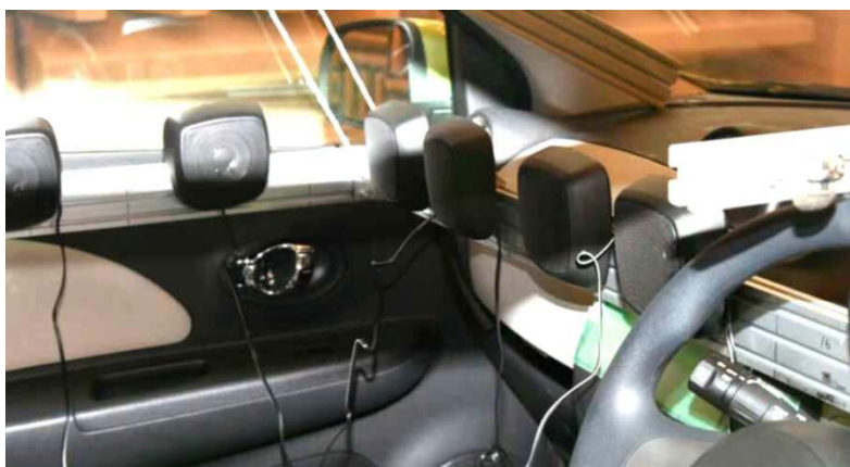
Fig. 4 Sound partition in vehicle interior with multiple speakers system
