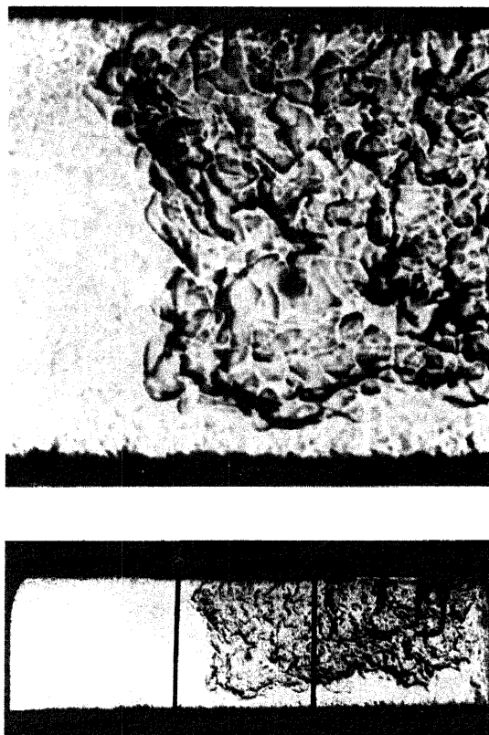
Fig. 4: Schlieren photograph of the turbulent, wrinkled reaction-sheet, spark-ignition engine flame (1). Lower photo shows the full square-cross-section engine combustion chamber; upper photo shows the center portion enlarged. Operating conditions: stoichiometric, propane fuel, 1400 rev/min, 0.5 bar inlet pressure.
