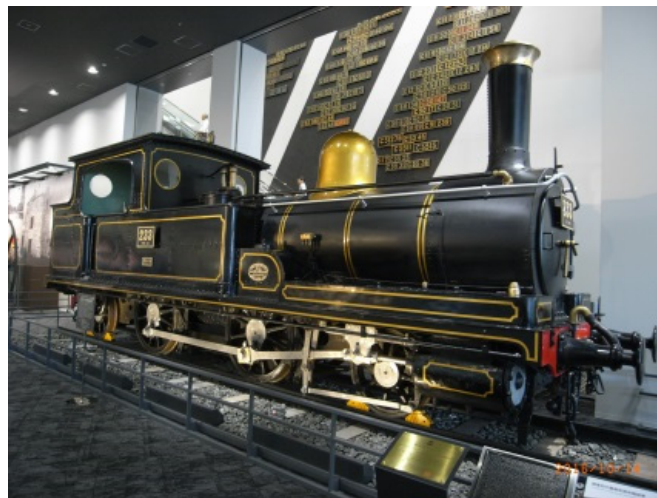
Fig.2 Class 230 No.233 Steam Tank Engine (Kyoto Railway Museum)
