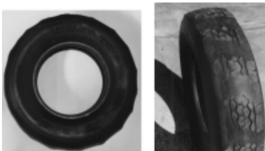
Fig. 2 Polygonal wear of tire
