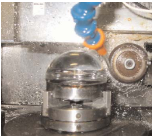
Fig.4 Mirror surface grinding of aspheric lens
