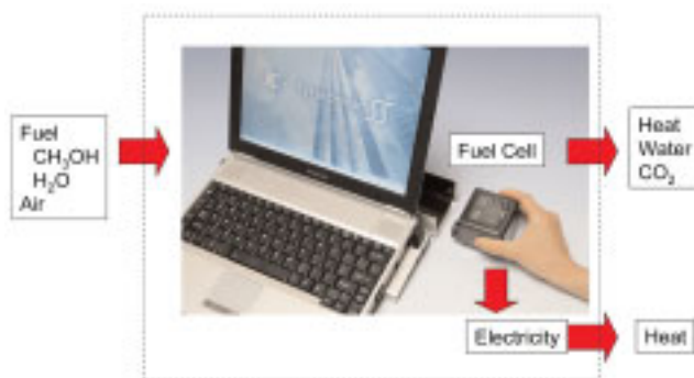
Fig. 1 Overall balance of material and energy in a DMFC for a portable equipment
