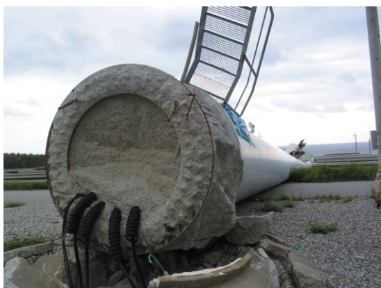
Fig. 3. Destroyed wind turbine by typhoon in Miyako-jima island, Okinawa
