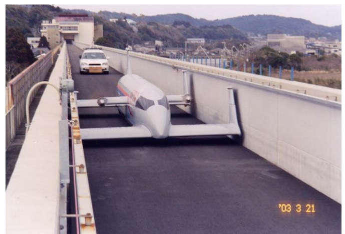
Figure 2. ART002 model cruise at 120km/h (Unmanned, 150km/h with zero-emission. Length:8.5m, Width:3.3m, Height: 1.7m, Weight:420kg, Engine: 5kW motor driven propeller x 2)
