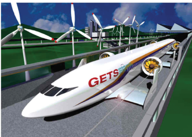
Figure1 Conceptual design of the Aero-Train. (500km/h cruise with 350 passenger by 3 coaches. Length:85m, Width:12m, Height:5m. Engine: 4 motor driven ducted fans. Electricity is from both side cable through special pantographs to motors)
