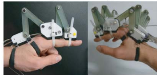
Figure 3. Power-assisted robot that passively moves paralyzed fingers by a wire-driven link mechanism
