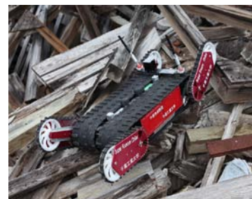
Fig1 Quince running over wooden rubbles
