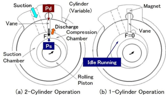
Fig.1 Illustration of variable cylinder mechanism
