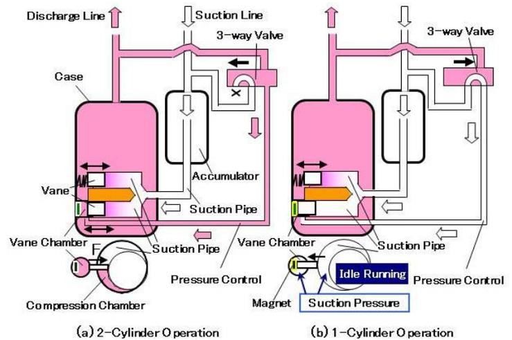
Fig.2 Switching operation of developed model
