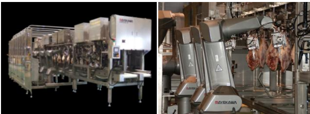
Figure 1 Automatic deboning robot system for pork thigh
