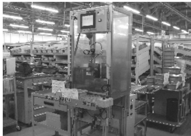
Fig. 4 Finishing equipment for small gear introduced in the gear production line
