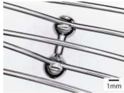
Fig. 2 shows a close-up of Laser micro-welded sections (on each temple)
