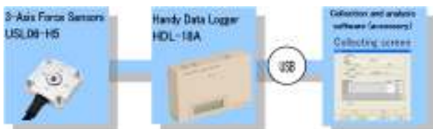
Fig.2 Measurement system structure
