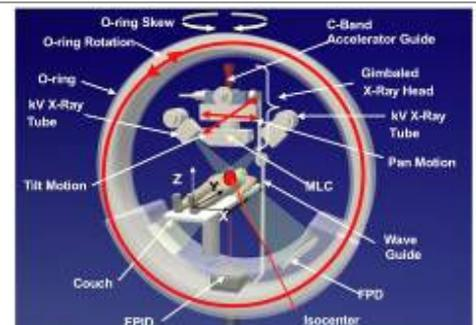
Fig. 3 Structure of the compact c-band accelerator
