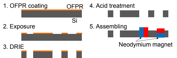
Fig.3 Fabrication process of on-chip robot.
