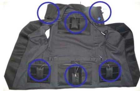
Fig.5 Vibro motors mounted at six places marked above in the vest
