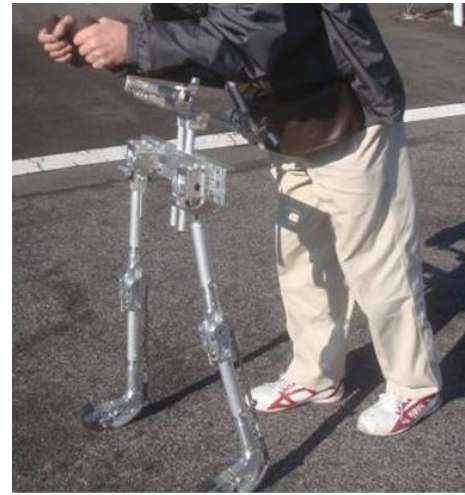
Fig.4 Legged assist walker
