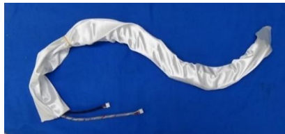
Fig. 5 Joint driving device with cloth cover
