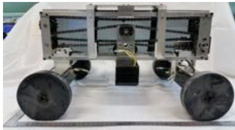
Fig. 5 Vehicle with WB variable changed unit and center of gravity moving unit
