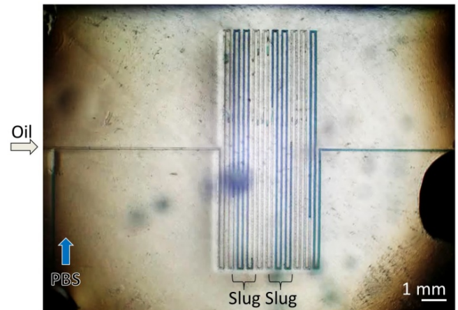
Fig. 2 Suppression of liquid mixture in a tube using slug flow
