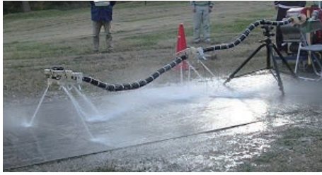
Fig.8 Result of Stable Float of Long Body by Water jet injection
