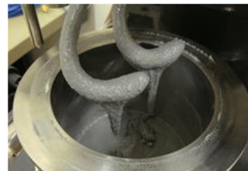
Fig. 2 Existing manufacturing method: Planetary Mixer.
