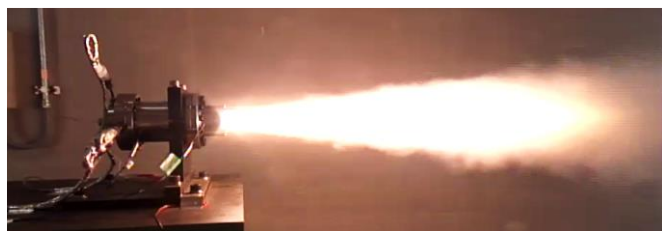
Fig.6 Burning test of solid rocket that used solid fuel kneaded by the peristaltic mixing conveyor
