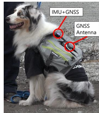
Fig.2 Cyber-enhanced rescue canine suit equipped with an IMU sensor, a GNSS receiver, and a camera with microphone.
