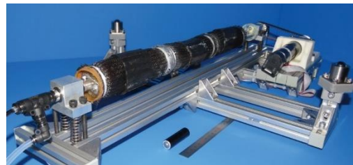
Fig. 2 Wave wheel mechanism using pneumatics [2]
