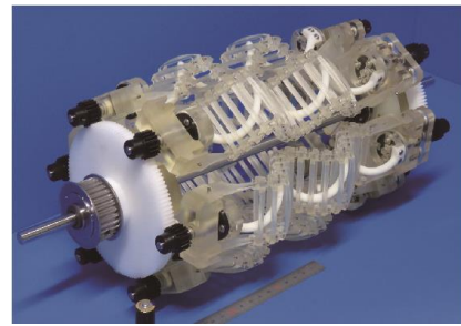
Fig. 5 Wave wheel mechanism using helical shafts [4]
