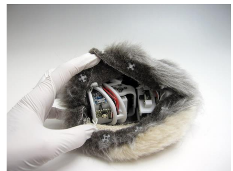
Fig. 3 Fur-covered skeletal robot
