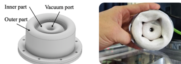
Fig. 1 Schematic drawing of double-layered UVG.
