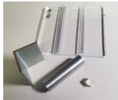
Fig. 4 Objects for gripping experiment. Top is the uneven acrylic plate for the adhesion experiment, and lower three pieces are metal angle, stainless steel pole, and tiny block.
