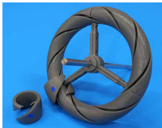
Fig.2 Slit structure to avoid interference with spokes
