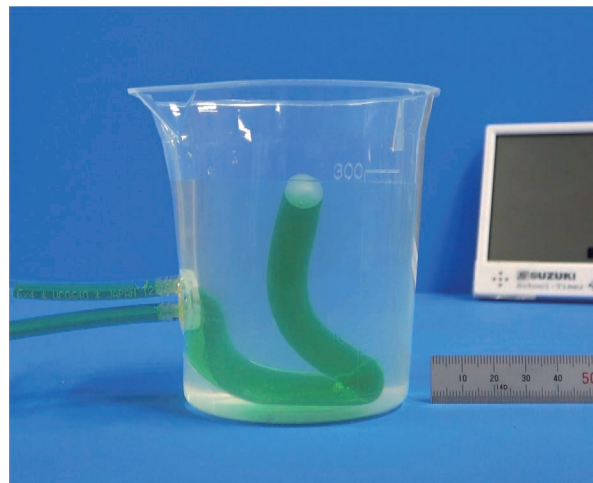
Fig.1 Tip growing mechanism with alginate gel tube
