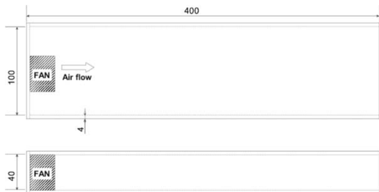
Fig. 10 1U size simplified experimental enclosure
