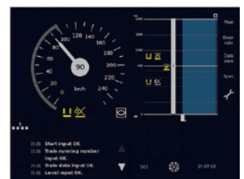
図3 ETCS の DMI (Driver Machine Interface)
